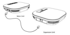
Connection Figure of Main Unit with Expansion Unit
